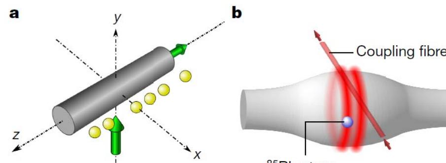
Figure 3 | Nanophotonic devices used for chiral coupling between light and quantum emitters.
